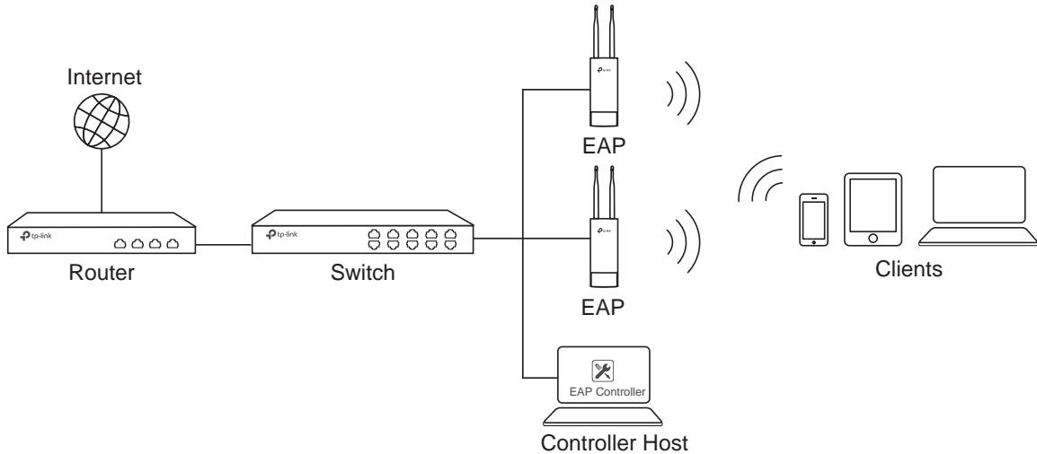
A computer running the EAP Controller software, which can be in the same or different subnet with the EAPs, is used to centrally manage the EAPs.
