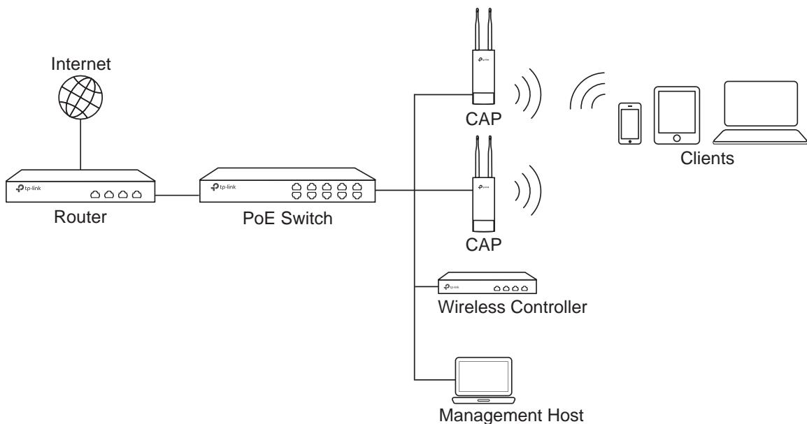
The wireless controller can be in the same or different subnet with the CAPs. And the management host is used to log in to the wireless controller to centrally manage the CAPs.
