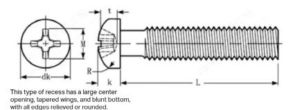
Screw Head Thickness k (mm) Screw Head Diameter dk (mm) Diameter ANSI B1.1 d(mm) max min max min 2.84 5.56 5.207 2.032 1.778 4# 6# 3.51 6.858 6.5 2.464 2.21 8# 4.17 8.179 7.772 2.921 2.667
