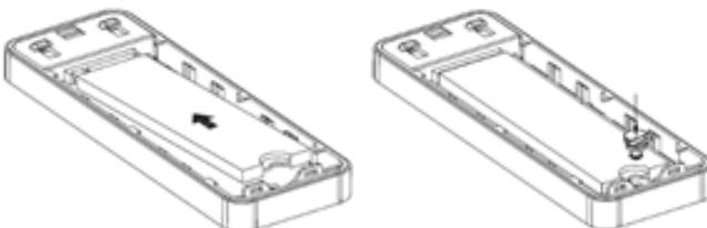
Step 3: Close the bottom cover, push as shown the direction of picture.
