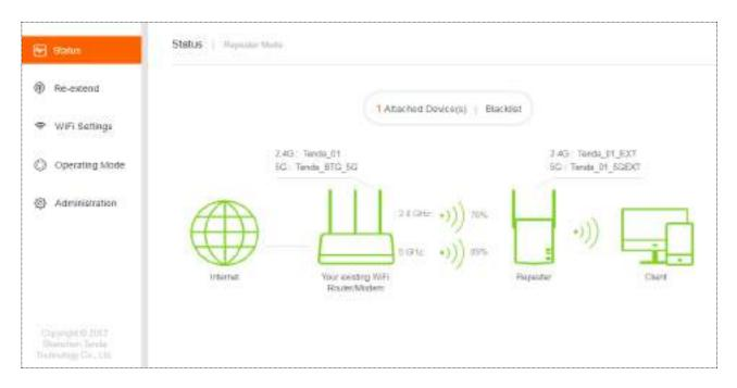
The internet connection status between the repeater and the upstream WiFi router/modem is shown using figures.
