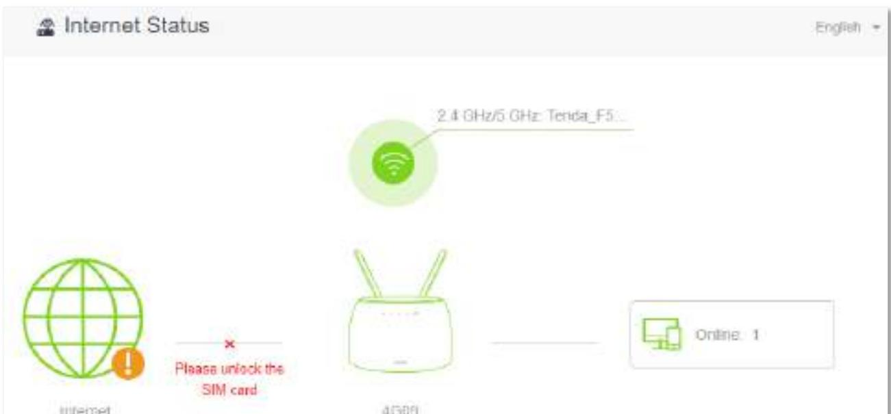
When a red cross and “No SIM card inserted” are shown between the Internet and the Router, ensure the SIM card is inserted properly.
