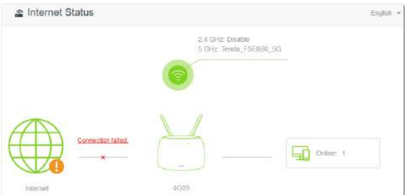
When “Please ensure that the cable between the Internet port of the router and the modem is properly connected” is shown on the page, ensure that the Ethernet cable between the WAN/LAN port of the router and the modem is connected properly. If the problem persists, contact the technical support for help.
