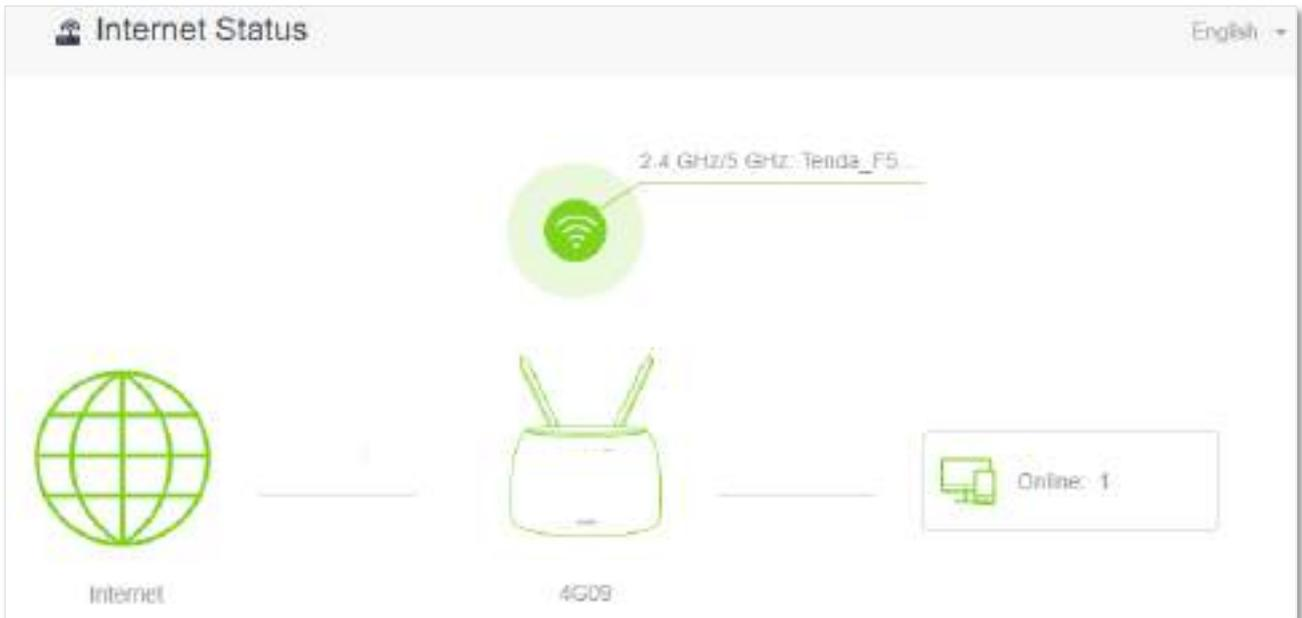
When a red cross and "**Connection failed.**" are shown between the **Internet** and the **Router**, it indicates that the internet connection is abnormal. Please click **Connection failed.** to navigate to the **Internet Settings** page and refer to the following scenarios and solutions.
